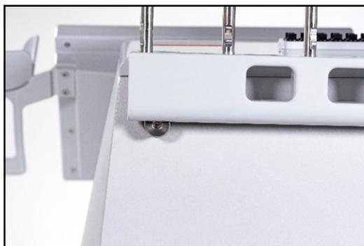
*Installing the vial rack*
