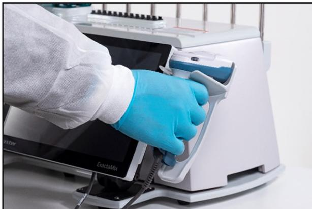
*Placing the barcode scanner*
