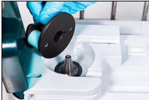
*Removing the pump rotor*
