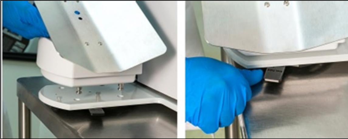
*Installing the load cell*
