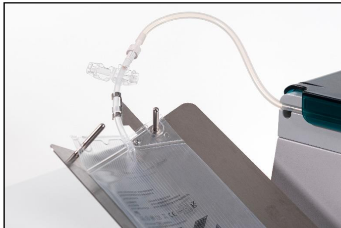
Attaching the calibration bag to the outlet tube and the load cell
